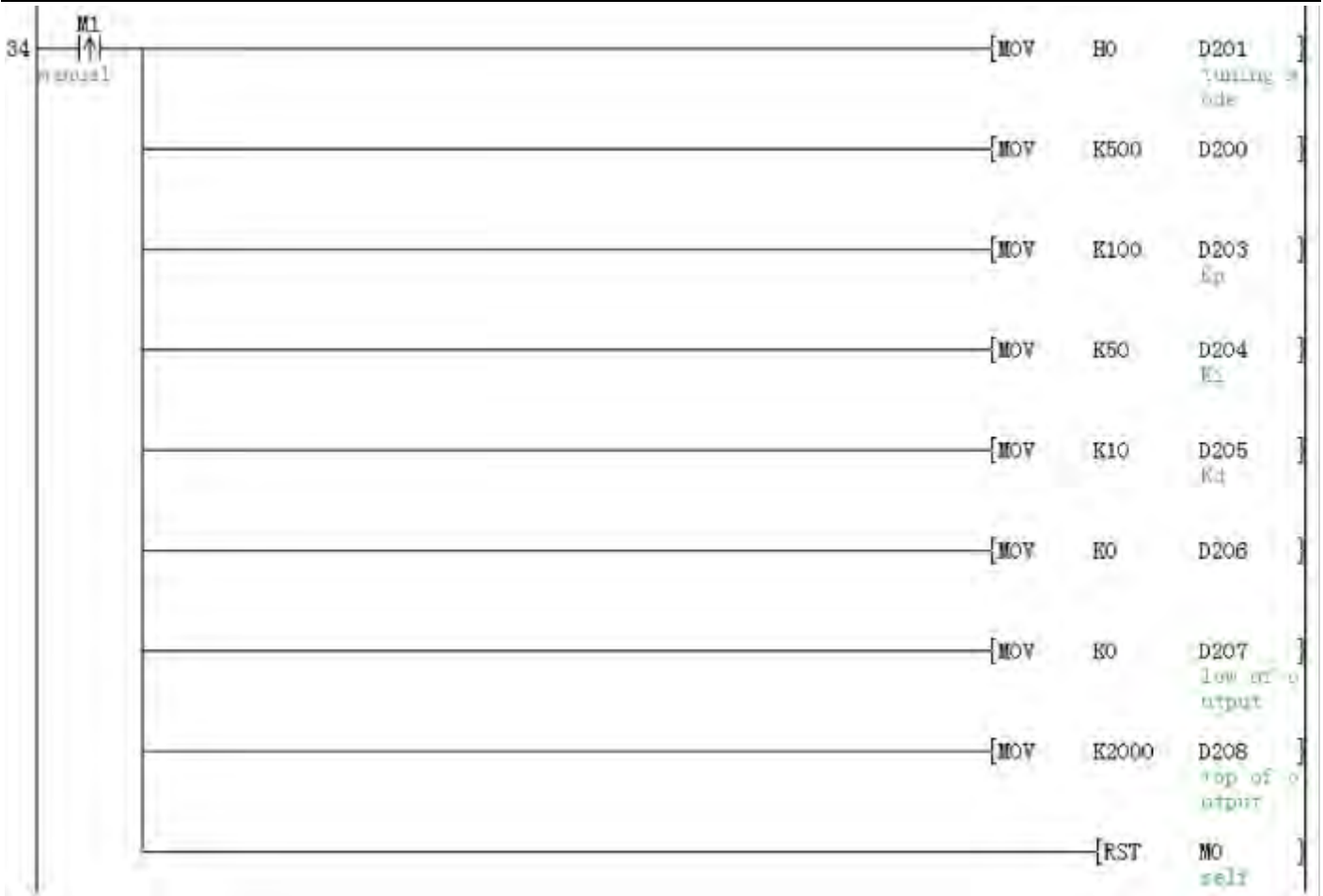
4) Trigger PID command by M0 or M1.
